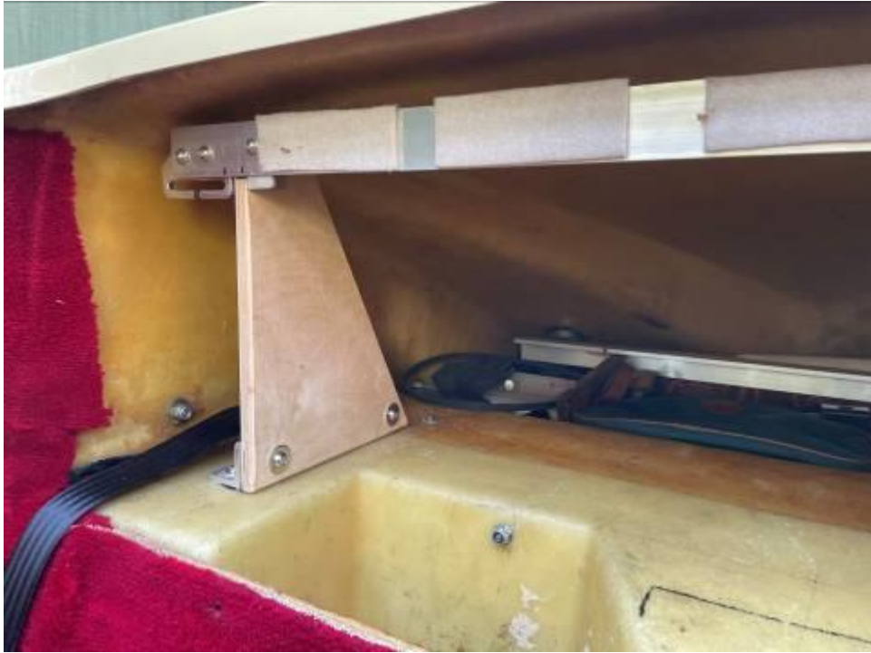
Seat belt guides fastened to transverse backrest support.
