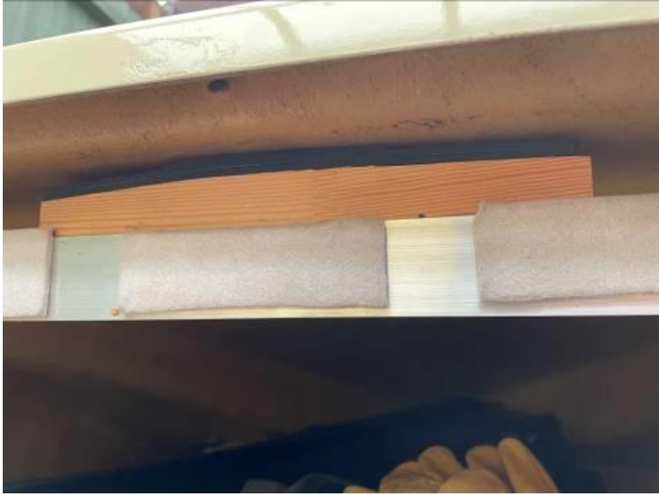
The body support block in positions.
