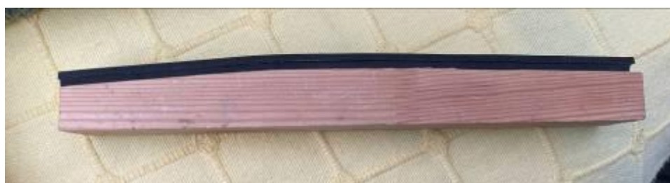
The rubber covered body support block.
