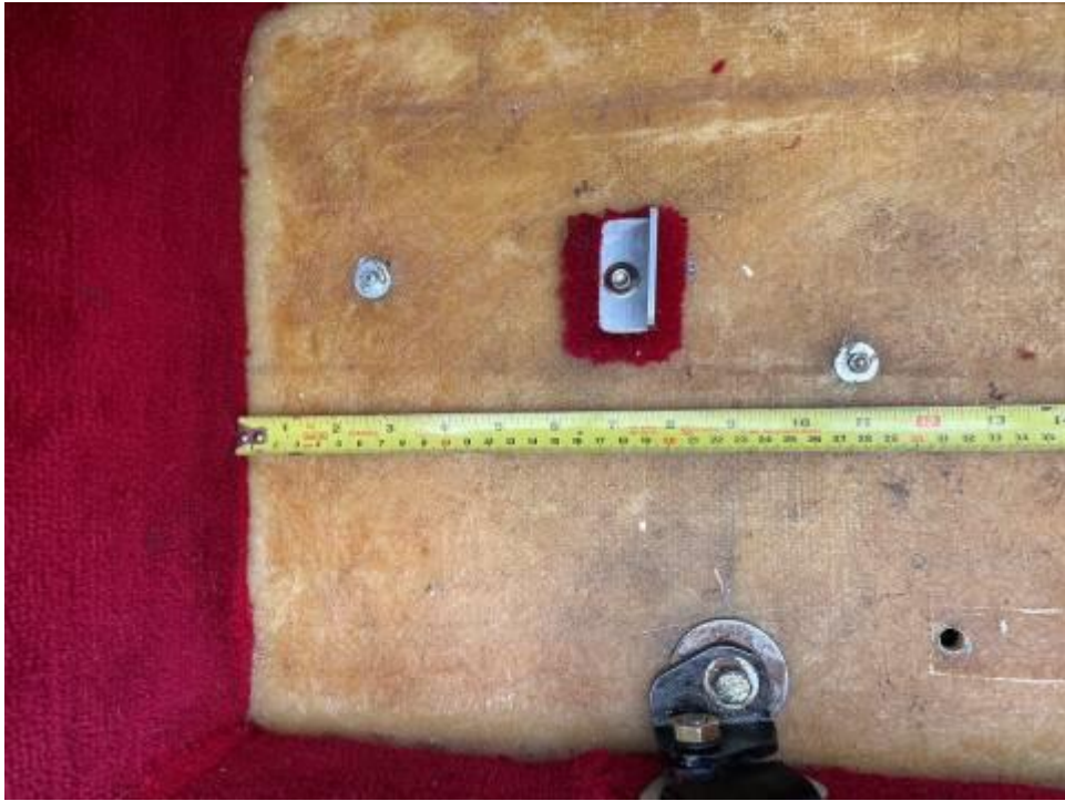
One of the 2" long equal aluminium angle pieces that locate the bottom of the backrest.
