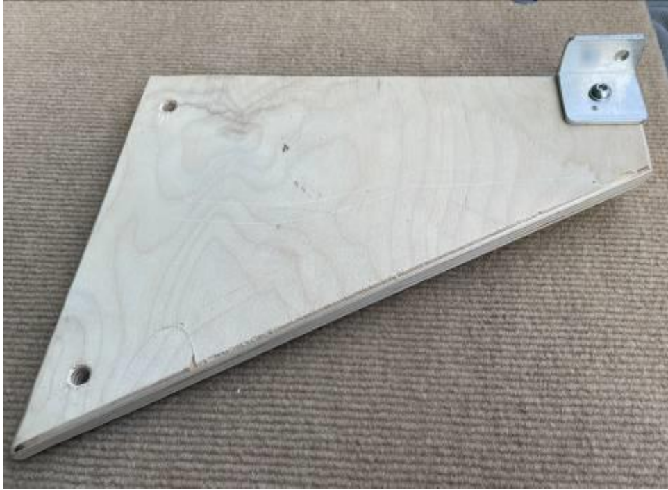
The brackets that support the transverse backrest support.
